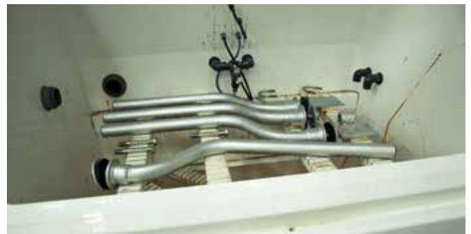
In-house testing of components at Coseley includes a 500-hour salt spray test in an Ascott cabinet that matches the most hostile road conditions encountered in winter months
